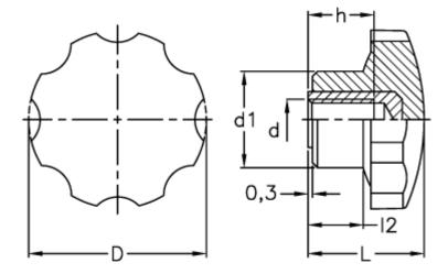
$$\begin{array}{ll} D & = 35 \\ d1 & = 19 \\ d \ 6H = M6 \\ h & = 12 \\ L & = 22 \\ l2 & = 10 \end{array}$$
